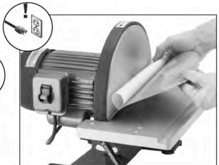
Figure 5. Sandpaper being slipped between the disc and table.
